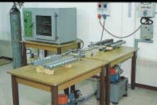
a bench for mechanical cycling of pressure transducers
