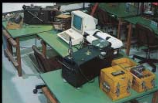
a bench for final test certification of pressure transducers
