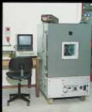
a climatic chamber: -85 \pm 180^{\circ}\text{C} for MIL-OML-ECC tests
