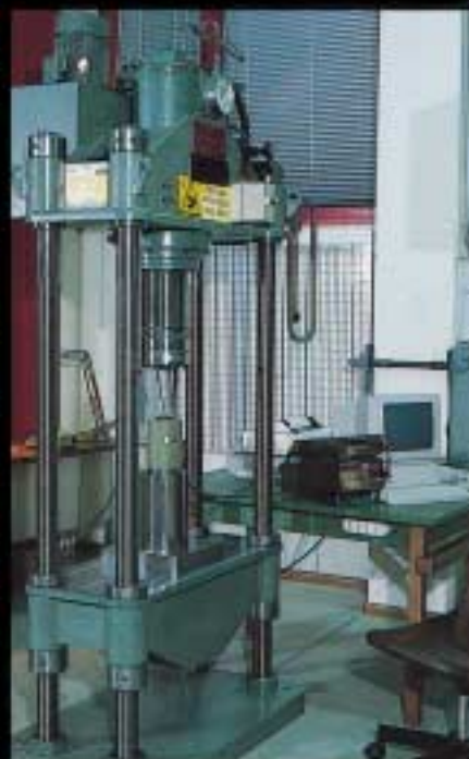
a bench for final test certification of load cells
