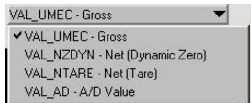
**VAL\_UMEC – Gross:** system displays the gross measurement in engineering units. Decimal point, if needed, is to be set using View→Decimal Point command. This measurement is obtained by transmitting to the system a @?R01 command with DSEnet protocol.
